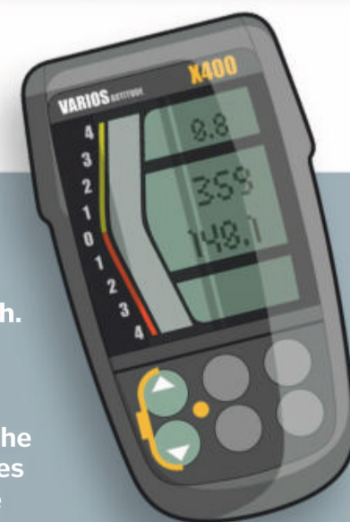
Variometers are most commonly used when navigating a thermal column
