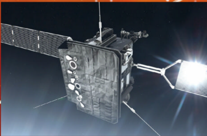
This artist's impression shows how the remote-sensing cameras look out through the spacecraft's sunshield
